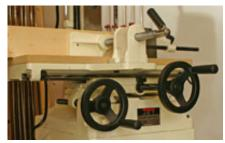
Large handwheels provide smooth, accurate control over the table movements.
